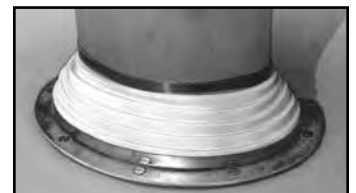
Finished Mast Boot
